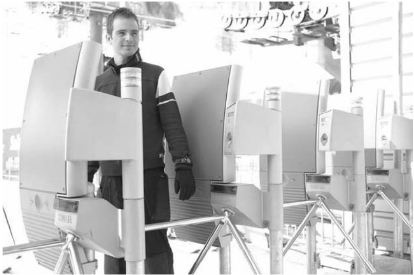
Figure 13.22 Contactless reader as access control and till device at a ski lift (reproduced by permission of LEGIC Identystems AG, CH-Wetzikon)
