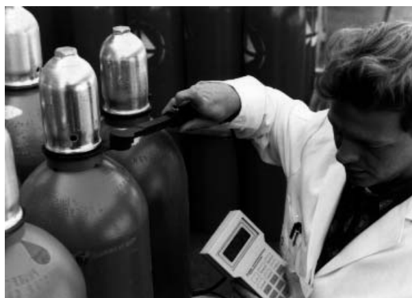
Figure 13.46 Identification of gas bottles using a portable reader. The reader (scemtec SIH3) is designed to function with transponders from different manufacturers (reproduced by permission of Messer Griesheim)
